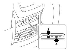
There are 2 USB ports (3 & 4) located on rear console plate, when the START/STOP Switch is in the ACC or ON/READY positions, the USB ports can provide 5V voltage serving as power outlets.
