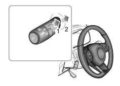
The MG Pilot system switch is located in the infotainment display. Enter the corresponding interface for driving assistance to turn the system ON/OFF. Operating the adaptive cruise control level to "RESUME" twice will switch the MG Pilot system to standby or active state.
