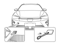
Your car is equipped with a towing eye (located at the front of the vehicle), which is used for fitting the towing hook in the tool kit. The tool kit is placed beneath the loadspace floor.
