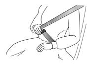
2 Insert the metal tab into the buckle until you hear a 'click', this indicates the seat belt is securely locked.
