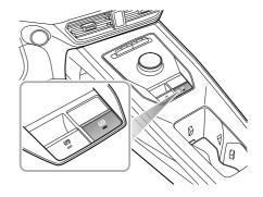
In some circumstances such as releasing the seat belt, switching off the power system or remaining static for a length of time, it will result in exiting the Auto Hold Parking state. At this time the electronic parking brake will be applied.
