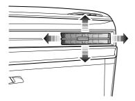
Slide the button in the centre of the louvres to the left or right to open or close the vent. Toggle it up and down, left and right to adjust the air direction.
