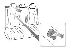
To increase the luggage space, the rear seat backrest can be folded fully forward. When folding the backrest completely, firstly insert the rear seat belt buckle into the corresponding slot, then fully lower (or remove) all head restraints, pull the respective control lever at the top of the seat backrest upwards and fold the seat backrest forward. To return the backrest to an upright position,
