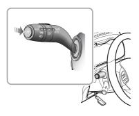
Having turned the lane assist system ON in the infotainment display, press the button at the end of the indicator stalk switch (as shown above) , the system will enter the standby or active state.
