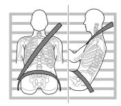
When wearing seat belts, the lap belt section should be positioned as low as possible across your hips. NEVER cross the abdomen. In the event of a collision, the lap belt can apply a force on the hips and reduce the possibility of
