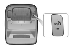
Note: The operation of eCall - SOS Emergency Assistance relies on cellular coverage and may be affected by signal outages or low signal strength.
