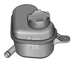
The cooling system should be checked weekly when the cooling system is cold and with the car resting on level ground. Open the bonnet and check the coolant level. If the coolant level is below the "MIN" mark, open the coolant expansion tank cap and top up coolant. The coolant level should not be higher than the "MAX" mark.
