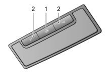
Press any one of buttons (2) to switch on the corresponding lamp, and press it again to switch the lamp off.
