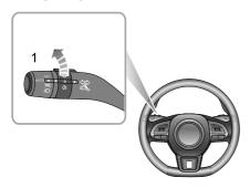
With the START/STOP Switch in the ON/READY position and the headlamps on, rotate the fog lamp switch to position I to turn on the rear fog lamps. The rear fog lamp indicator illuminates in the instrument pack when the rear fog lamps are on.
