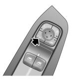
Note: For vehicles equipped with power folding exterior mirrors, the power folding function of exterior door mirrors can also be realized by touching the mirror fold/unfold switch on the entertainment display screen.
