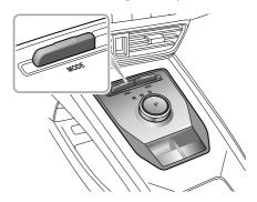
The driver can select three driving modes by operating the MODE switch:
