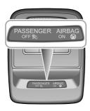
The passenger airbag status light is located in the roof mounted interior lamp assembly. The shape of the lamp assembly varies according to the configuration of the vehicle.
