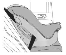
It is recommended that children should always be seated in the rear of the vehicle in a child restraint or restraint system, and fixed with 3 point, lap diagonal seat belts.
