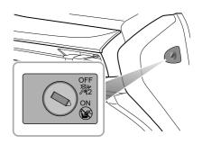
The passenger airbag switch is located in the right fascia panel end cover trim. Insert the key and rotate the switch to the on or off position to enable or disable the passenger airbag.
