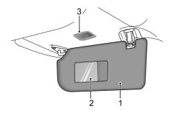
Sunvisor (1), vanity mirror (2) and vanity mirror light (3) are arranged on the roof ahead of both the driver and the front passenger.
