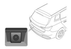
A rear parking camera is fitted between the license plate lamps. When reverse gear is selected, the camera will
