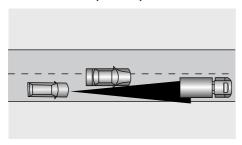
If the vehicle ahead changes lanes, but does not drive into the lane completely, the adaptive cruise control system may be unable to detect the vehicle.
