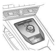
The shift control knob defaults to the intermediate steady state position, there are two unsteady positions clockwise and counterclockwise, the shift control knob will return to the intermediate steady state position once released.
