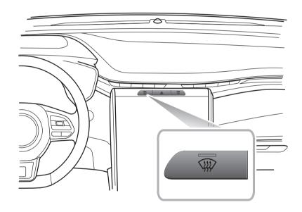
Press this button to operate the defrost/demist function, the indicator will illuminate. The system will automatically set itself to a preset temperature and blower
