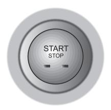
The keyless START/STOP Switch is located in the fascia to the right of the steering column. It is a push button style switch. To operate the switch the smart key must be inside the vehicle.
