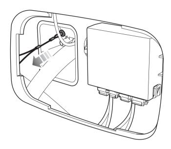
Pull the release cable handle, remove the connector plug whilst maintaining tension on the cable this will release the locking device.
