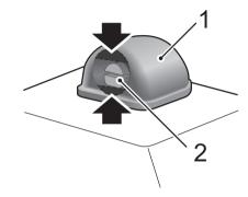
Operate the washers periodically to check that the nozzles are clear and properly directed.
