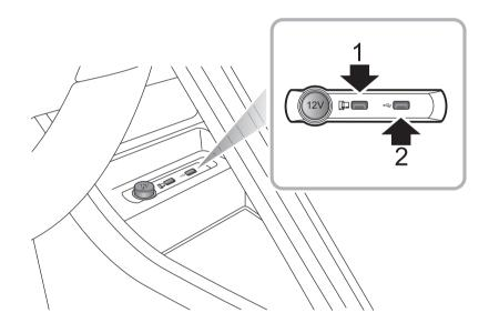
The I2V front console power socket is located in the front of console. When the START/STOP Switch is in the ACC or ON/READY positions, it can be used as a power supply.
