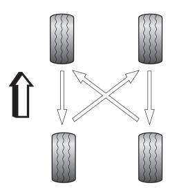
Note: Directional tyres (identified by the arrow on the tyre sidewall) CANNOT be swapped diagonally or from side to side.
