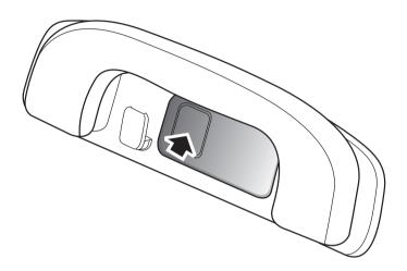
The rear courtesy lights are located on the left and right sides of interior roof panel. Press the lamp lens as indicated in the diagram to switch on the rear courtesy lights. Press it again to switch off the lights.
