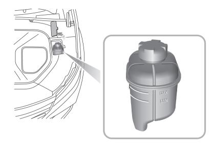
The cooling system should be checked weekly when the cooling system is cold and with the car resting on level ground. Open the bonnet, remove the coolant expansion tank trim cover and check the coolant level. If the coolant level is below the "MIN" mark, open the coolant expansion tank cap and top up coolant. The coolant level should not be higher than the "MAX" mark.
