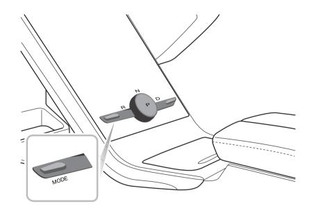
The driver can manually select four driving modes by operating the MODE switch on the electronic shifter in
