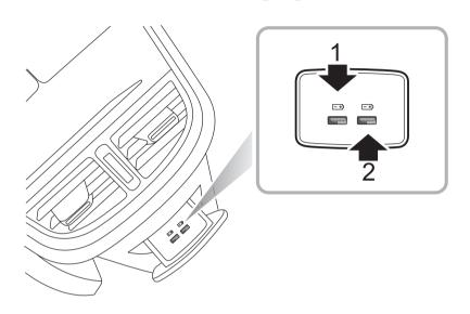
Note: Use of the rear console USB port when the vehicle is not in READY mode will consume battery power, extended use will cause premature discharging of the vehicle battery, and the vehicle may be prevented from being switched into READY mode.
