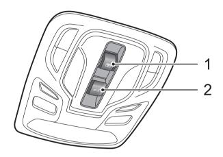
When the START/STOP Switch is set to ACC or ON/READY, you can operate the sunroof.
