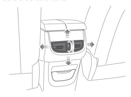
Rotate the thumb-wheel up or down to open or close the vents.
