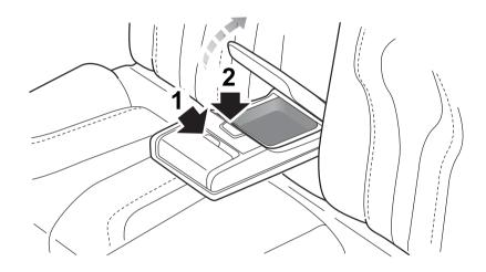
Fold forward to open the rear armrest. Press button I to open the cup holder. Press button 2 to open the storage box in the rear of the armrest.
