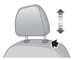
The head restraint is designed to prevent rearward movement of the head in the event of a collision or
