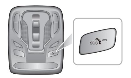
indicator will be extinquished or flash slowly if a fault is detected. Faults detected during the self-test will be displayed on the vehicle's message centre.
