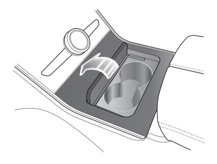
The centre console cup holder is situated at the front end of the centre console armrest assembly. Press the cover of the cup holder to open.
