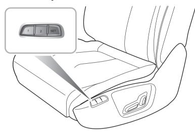
Vehicles with the memory function can provide a greater set of personalized settings for driving: this includes adjustment and memory of seat position and exterior rearview mirror angle (allowing the setting and saving of personalized settings for two drivers).
