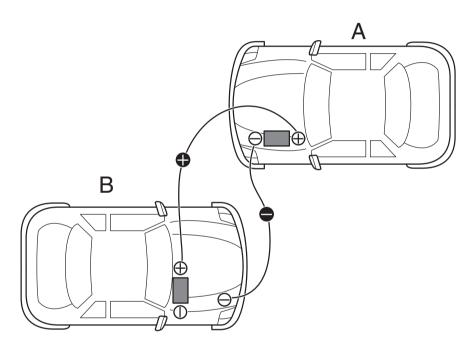
Depending on the configuration of the vehicle, the location of the battery is different. The battery for two-wheel drive vehicle is located at the rear right side of the front compartment, while the battery for four-wheel
