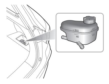
The cooling system should be checked weekly when the cooling system is cold and with the car resting on level ground. Open the tailgate, remove the coolant expansion tank trim cover and check the coolant level. If the coolant level is below the "MIN" mark, open the coolant expansion tank cap and top up coolant. The coolant level should not be higher than the "MAX" mark.
