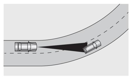
When turning at an intersection or following a vehicle into, or out of a curve, the adaptive cruise control system may be unable to detect the vehicle ahead, even if it is in the same lane, it is possible the system may detect a vehicle in another lane.
