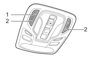
Press switch I to turn on the front interior lamps. Press again to turn off.
