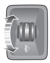
The headlamp leveling can be adjusted as per the following table according to the vehicle load.
