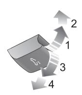
Push the sunroof glass switch upward to the 1st position (1) and hold. The sunroof will tilt open. You can stop the movement of the sunroof at any time by releasing the switch. Push the glass switch with slightly harder force to move the switch to its 2nd position (2) and then release, the sunroof will automatically open completely.
