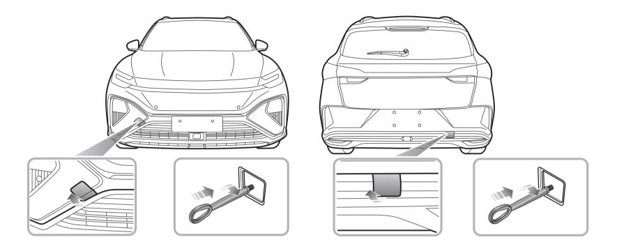
Your car is equipped with 2 towing eyes (located at the front and the rear of the vehicle), which are used for fitting the towing hook in the tool kit. The tool kit is placed beneath the loadspace floor.
