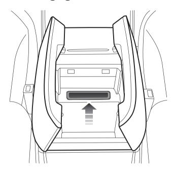
The wireless charging area is located in the front storage box. The charging function is enabled when the START/STOP Switch is placed in the ACC/ON/READY positions. Open the storage box cover and place the phone vertically in the card slot. The charging coil of the mobile phone should be facing front. This can be used for wireless charging.
