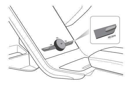
The driver can manually select three energy regeneration levels by operating the REGEN switch on the electronic shifter in the infotainment display.
