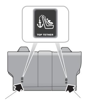
3 To fasten the top tether strap of the child restraint system, route the tether strap under the head restraint and attach to the anchorage hook, being careful not to twist the strap. If not using ISOFIX lower anchorages, using the seatbelt, complete the installation in line with the child restraint manufacturers instructions.
