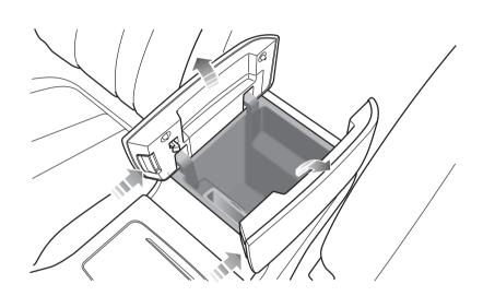
Press the buttons to the front of each cover and lift to open the cover (as indicated by the arrow), Push the cover down to close it.
