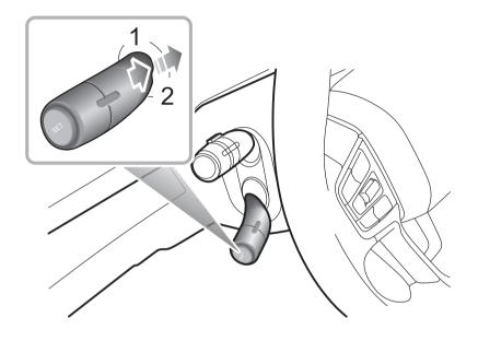
After turning on the adaptive cruise control system, operating the adaptive cruise control level to "RESUME" twice will switch the traffic jam assist system to standby or active state.
