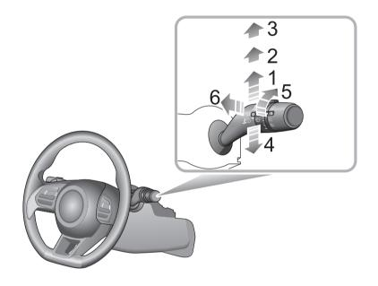
The wipers and washers will only operate when the START/STOP Switch is in the ON/READY position. Operate the lever to select different wiping modes:
