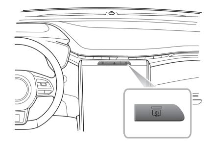
Press the Heated Rear Window Button to switch the function on or off. The button indicator illuminates when the function is on, and is extinguished when the function is off. The heated rear window features a timer function and will automatically switch off after a preset time. To continue to use the heated rear window, operate the button again.
