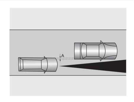
When driving behind a vehicle that is only partially overlapping your vehicle, 'A' in the graphic, the adaptive cruise control system may be unable to detect anything.
