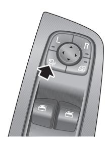
While unlocking/locking the vehicle, the exterior door mirrors will be deployed/folded automatically.
