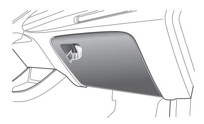
To open the glove box, pull the handle on the glove box cover (as indicated by the arrow). The glove box light will automatically illuminate.
