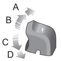
Each window switch is designed as a 2 stage switch. Press the window control switch  $(2 \sim 5)$  to the first position (C) to lower the window; and lift the switch to the first position (B) to raise. The window will stop moving as soon as the switch is released. Release the switch and the window stops.
