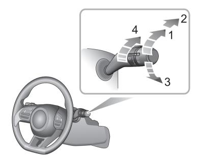
The rear wipers and washers will only operate when the START/STOP Switch is in the "ON/READY" position. Rotate the rear window wiper switch to your desired selection:
