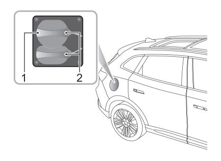
After charging, refit the waterproof plug covers, close the charging port door, push the door fully home until the latch locates.
