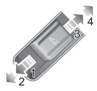
Push the sunroof glass switch backward to the 1st position (3) and hold. The sunroof will slide open. You can stop the movement of the sunroof at any time by releasing the switch. Push the glass switch backward with slightly harder force to move the switch to its 2nd position (4) and then release. The sunroof will automatically open fully. You can stop the movement of the sunroof at any time by pushing the switch backward again.
