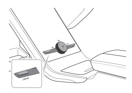
The driver can manually select five driving modes by operating the i-Drive switch on the electronic shifter in the infotainment display: WINTER Mode, ECO Mode, NORMAL Mode, SPORT Mode, SPORT+ Mode.
