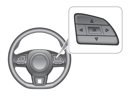
The instrument pack operation buttons are located in the RH steering wheel multifunction switch pack.
