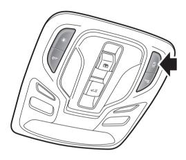
Press the button indicated in the picture to turn on or turn off the automatic function.
