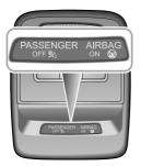
When the switch is turned to the OFF position, the OFF indicator light ( located in the PAB display panel in the lamp assembly ) illuminates, this indicates that the passenger airbag is disabled.
