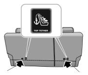
3 To fasten the top tether strap of the child restraint system, route the tether strap under the head restraint and attach to the anchorage hook being careful not to twist the strap. If not using ISOFIX lower anchorages, using the seatbelt, complete the installation in line with the child restraint manufacturers instructions.
