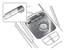
The driver can operate the BATTERY switch to display the energy management interface in the infotainment system.
