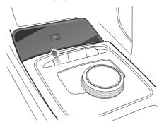
The wireless charging area is located in the front storage box. The charging function is enabled when the START/STOP Switch is placed in the ACC/ON/READY positions. Open the storage box cover and place the phone vertically in the card slot. The charging coil of the mobile phone should be facing front. This can be used for wireless charging. Note: Only one mobile phone can be charged at a time.
