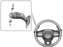
Move the lever down to indicate a LEFT turn (1). Move the lever up to indicate a RIGHT turn (2). The corresponding GREEN indicator lamp in the instrument pack will flash when the turning signal lamps are working.
