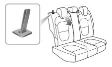
To increase luggage space, the rear seat backrest can be fully folded forward. When folding the backrest, first fully lower (or remove) all the rear seat head restraints, and then pull up the backrest unlock straps on both sides respectively and fold the seat backrests forward.
