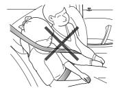
As children grow and become older/larger it will get to the stage when they no longer require child seat restraints. At this point they will require use of the vehicle standard seat belt. Please ensure the seat belt is correctly positioned on the body of the child.
