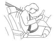
The diagonal section of the seat belt should pass across the chest as normal, the lap section of the belt should pass below the belly, low and snug on the hip bones. NEVER position the belt on or above the belly.
