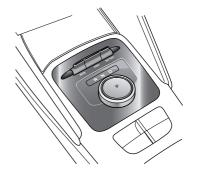
The shift control knob is in the intermediate steady state position, and there are two unsteady positions clockwise and counterclockwise, that is, the shift control knob will return to the intermediate steady state position once released.
